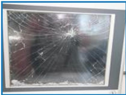
There were two incidents nine days apart where the Human/Machine/Interface (HMI) in the workstations were destroyed. The cost to replace the units was \$4,000 each, but the larger issue was expressed by the Safety Director, "That could have been an employee's head."
