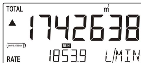
Fig. 4: Example of low-battery alarm
